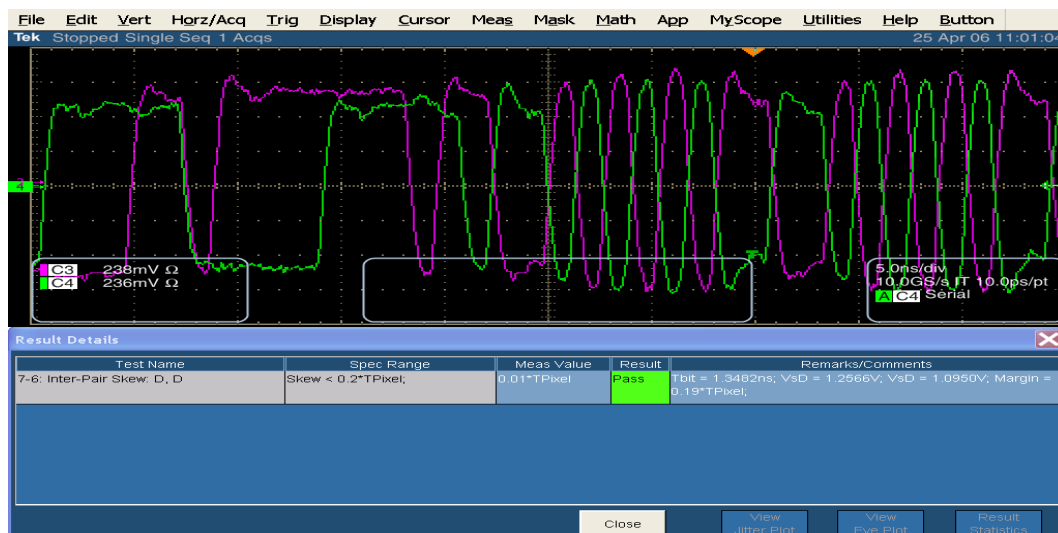
Figure 11 Data-Data inter-pair skew testing
